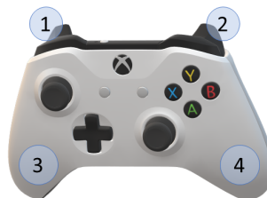
Figure 6.3: Microsoft Xbox One wireless controller, showing position of embedded trigger (1,2) and palm (3,4) ERM motors, and button layout.
