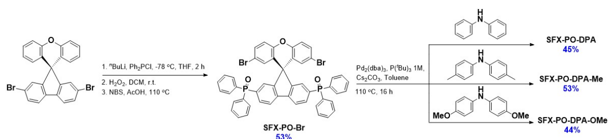
Scheme 1. Synthetic routes for SFX-PO-Br -starting material and three studied emitters: SFX-PO-DPA , SFX-PO-DPA-Me and SFX-PO-DPA-OMe .
