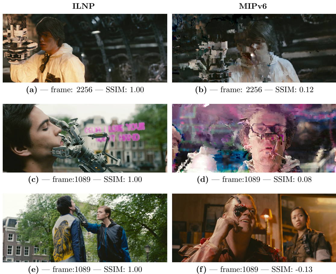
Figure 7.7: A series of frames captured after converting the received MPEG-TS files to raw YUV 4:2:0 files were used for analysis using VQMT. Images on the left column are frames captured from ILNP results. Images on the right column are frames captured from MIPv6 runs. (a) and (b) are the 2256th frame of the recorded clip. Frame (b), from the MIPv6 result, shows clear block noise and overall delay in image transition. (c) and (d) are the 1089th frame into the clip. Frame (d) from MIPv6 shows clear colour noise and block noise. Note that the part of the robotic arm with a needle similar to the one seen in (c) is visible, which is from the expected frame. The more dominant image in frame (d) is a man with glasses from the previous scene. (e) and (f) are the 1325th frame — they were mismatched. Frame (f) is visually not impaired, but it is not the expected frame at that time, which should be what (e) shows. Upon playing back the MPEG2-TS file, at the same timecode, frame (e) was displayed with the ILNP clip, but for the MIPv6 clip, the player displayed the identical frame shown in (f) for multiple seconds.
