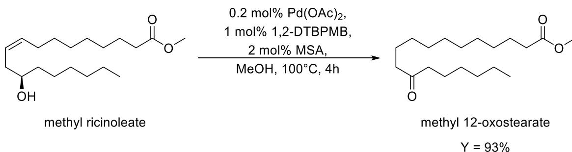
Figure 59: Pd/1,2-DTBPMB mediated double bond isomerization of methyl ricinoleate. 205
