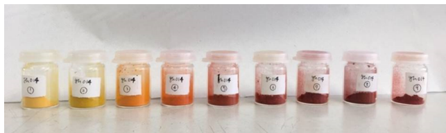
Figure 5. Photograph of halide substituted samples, \text{MXDBiI}_{5-x}\text{Br}_x .
