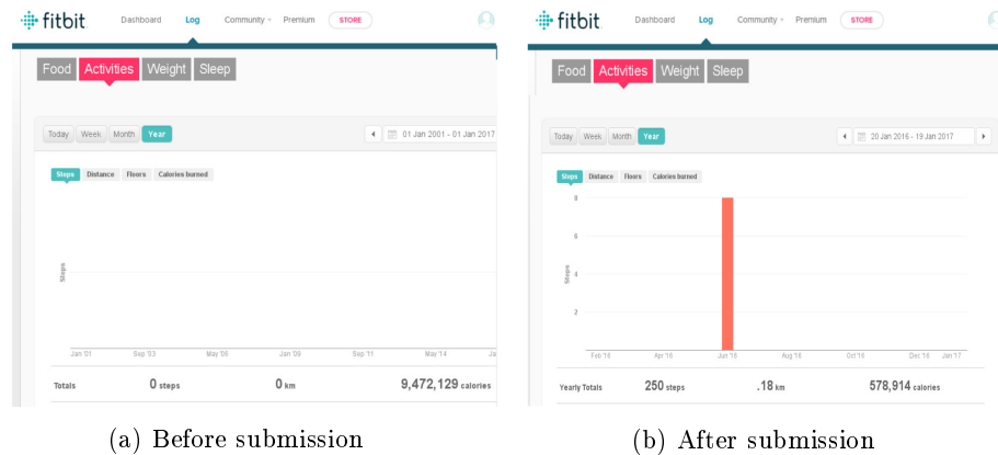
Fig. 9: The result of replaying data from another Fitbit tracker to a different tracker ID. Fig. 9a shows the Fitbit user activity screen before the replay attack, and Fig. 9b shows the results after the message is formed by changing the tracker ID, and submitted to the server.
