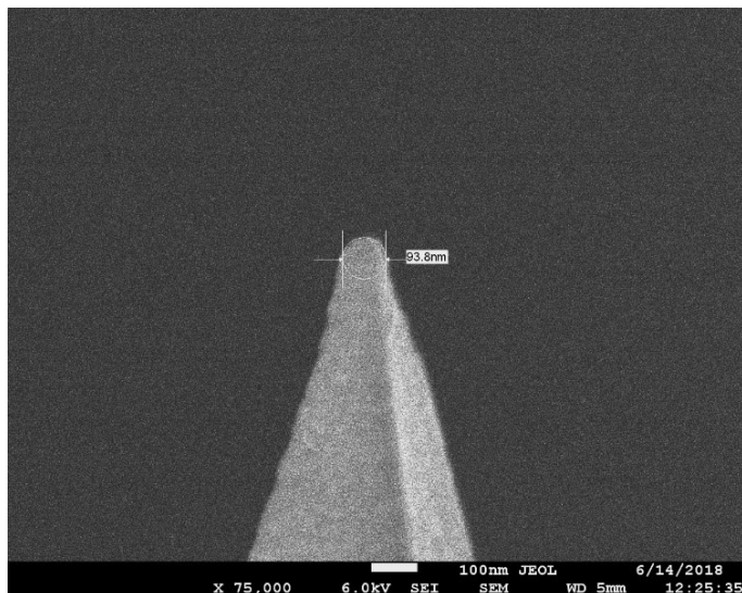
Fig. S4. SEM image of the CSG10/Au tip used in measurements.
