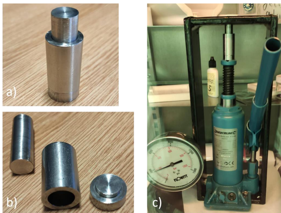
Figure 9.6. a, b) Photo of the stainless-steel metal mould. c) Photo of the PMMA heat moulding process using the bottle jack and the metal mould.
