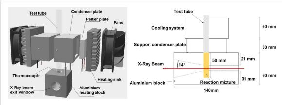
Figure 3. Schematic description of in-situ PXRD set up for investigation of heterogenous catalysts for biodiesel production.
