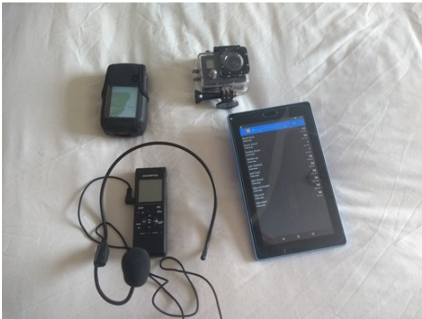
Figure 1. Equipment used during observer trips (clockwise from top left). The Garmin eTrex20x, the Campark Xtreme II UHD 4K action video camera, the Activity logger application on a handheld tablet, and the Olympus VN-741PC digital voice recorder.
