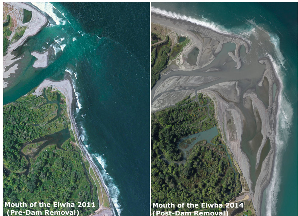
Fig. 6 The mouth of the Elwha River, Olympic National Park, WA, USA, in 2011 and 2014. The former shows the effect of dams upstream reducing sediment deposition. The latter shows that the river has returned to its natural state with the formation of sedimentary features and reinstatement of natural processes following removal of the dams (© US National Park Service)
