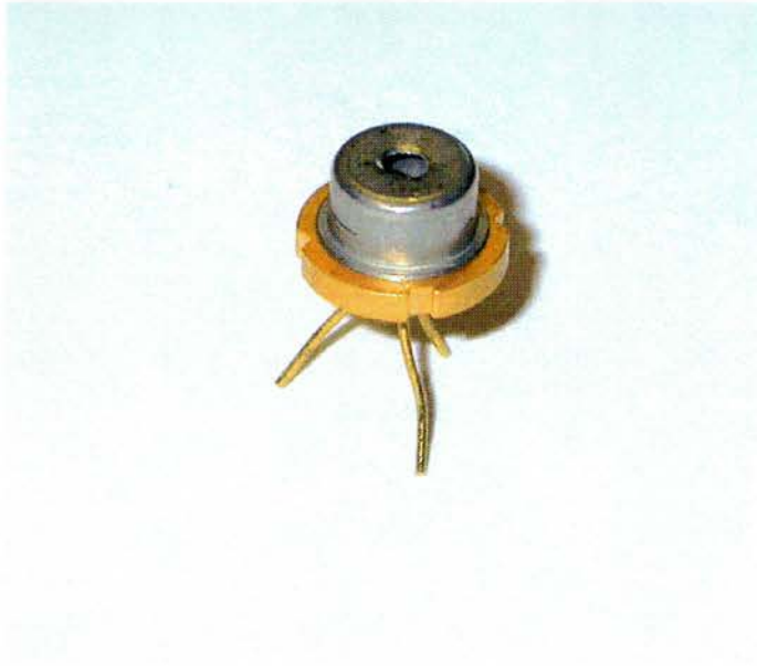
Fig. 1.2: A commercial diode laser in a 9.2mm transistor can.
