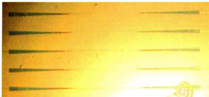
Fig. 8.6: The SU8 deep etch mask (appears green) prior to the insulation step. The taper and narrow waveguide region is clearly shown. (The chip will be cleaved on a line through the middle of the picture seen here, creating two sets of devices).
