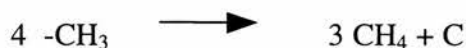
Scheme 1 Proposed mechanism for the pyrolysis of methyl groups in an inert atmosphere.
