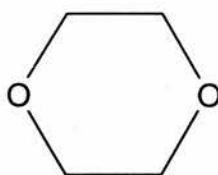
Figure 4 Structure of 1,4-dioxane. Note the high symmetry giving only one distinct carbon species and one oxygen species.
