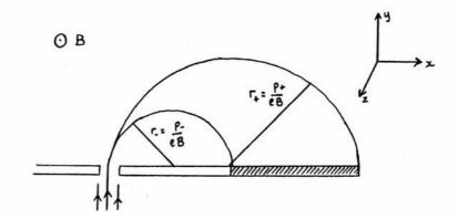
A beam of electrons with momentum in the y-direction lying in some (possibly unbounded) range  $\Delta p$ , say, enters the magnetic field. The particles are deflected according to [Clemmow 1973 p253,eg]
