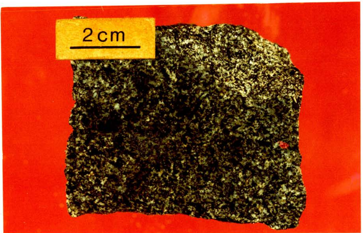
Plate 4.26 Hand specimen of melanocratic, fine-grained quartz-monzodiorite, RM89.
