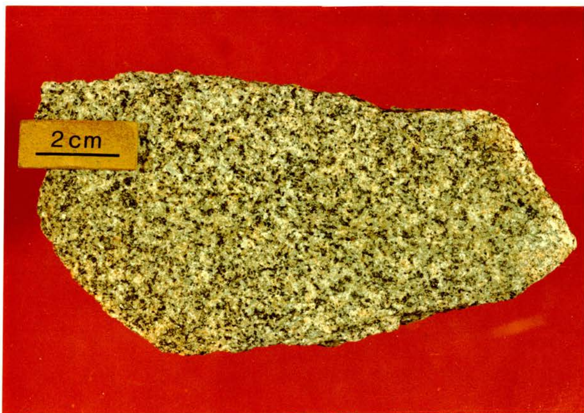
Plate 4.31 Hand specimen of mesocratic, fine grained monzogranite, RM112.
