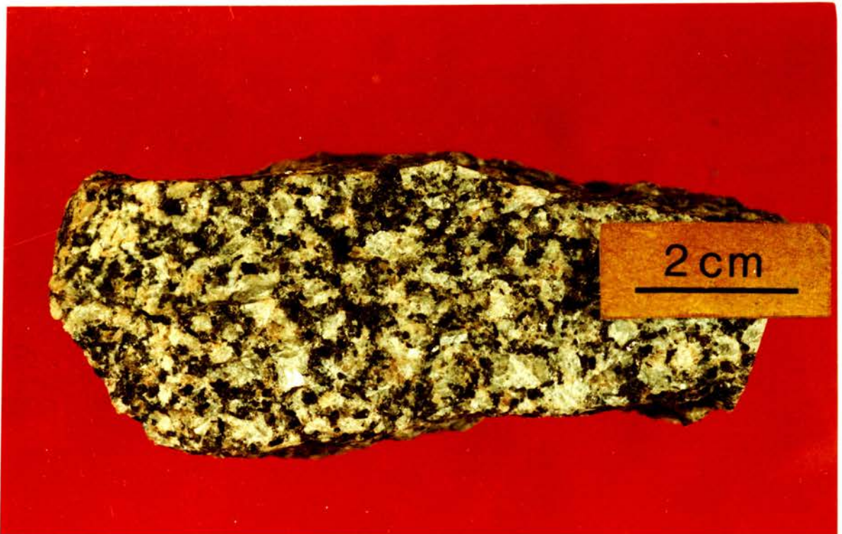
Plate 4.30 Hand specimen of leucocratic medium-coarse grained granodiorite, RM51.
