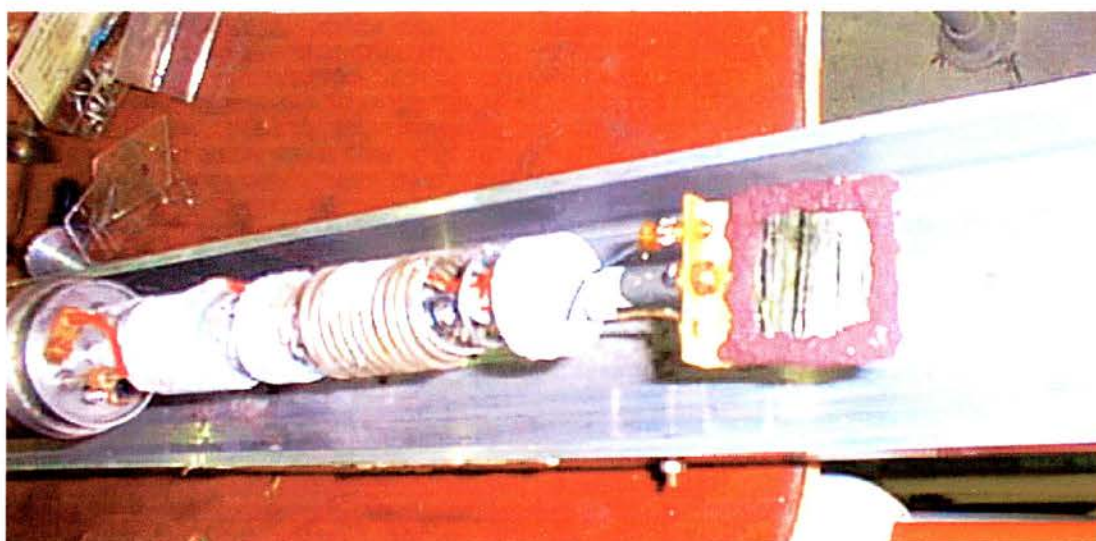
Figure III- 8 : An amorphous sample mounted on the MuSR dilution fridge showing the orientation of the ribbons and the surrounding haematite mask.
