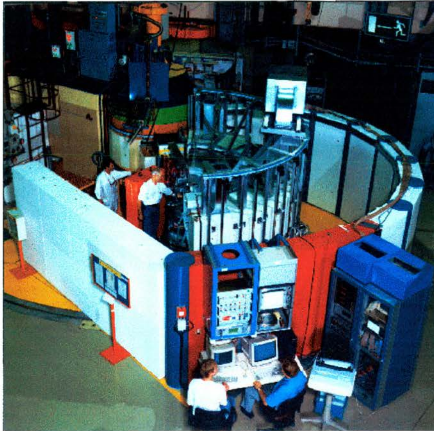
Figure V- 1 : Picture of the D20 instrument showing the impressive PSD detector bank covering a very wide range of 2\theta angles.
