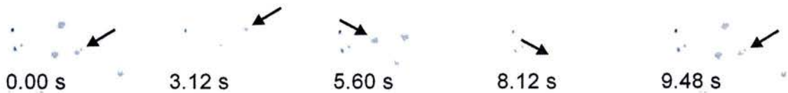
Figure 6.8: Rotation of three 1 \mu\text{m} diameter silica spheres in an l = 3 interference pattern. One of the spheres is tracked with an arrow.
