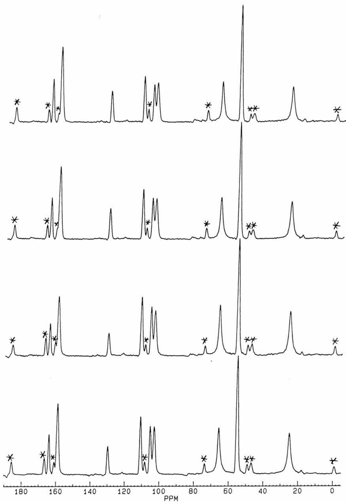
Figure 5.50. ^{13}\text{C} CP/MAS spectra for butane-1,4-diyl bis(3,5-dimethoxybenzoate) at different temperatures. Temperatures are from top to bottom: 270, 246, 222 and 190 K. Spinning sidebands (at 7 kHz) are asterisked.
