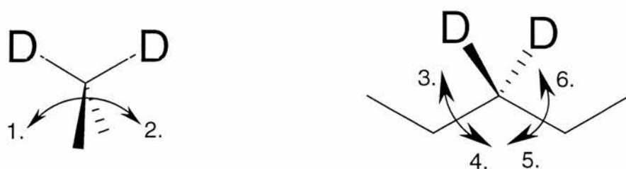
Figure 3.16. The origin of the six-site conical motion. Two sites are generated by libration of the chain about its axis (left), or equally, by a simultaneous rotation of the two bonds in different directions. The other four sites are obtained by rotations of the two C-C bonds in both directions (right).
