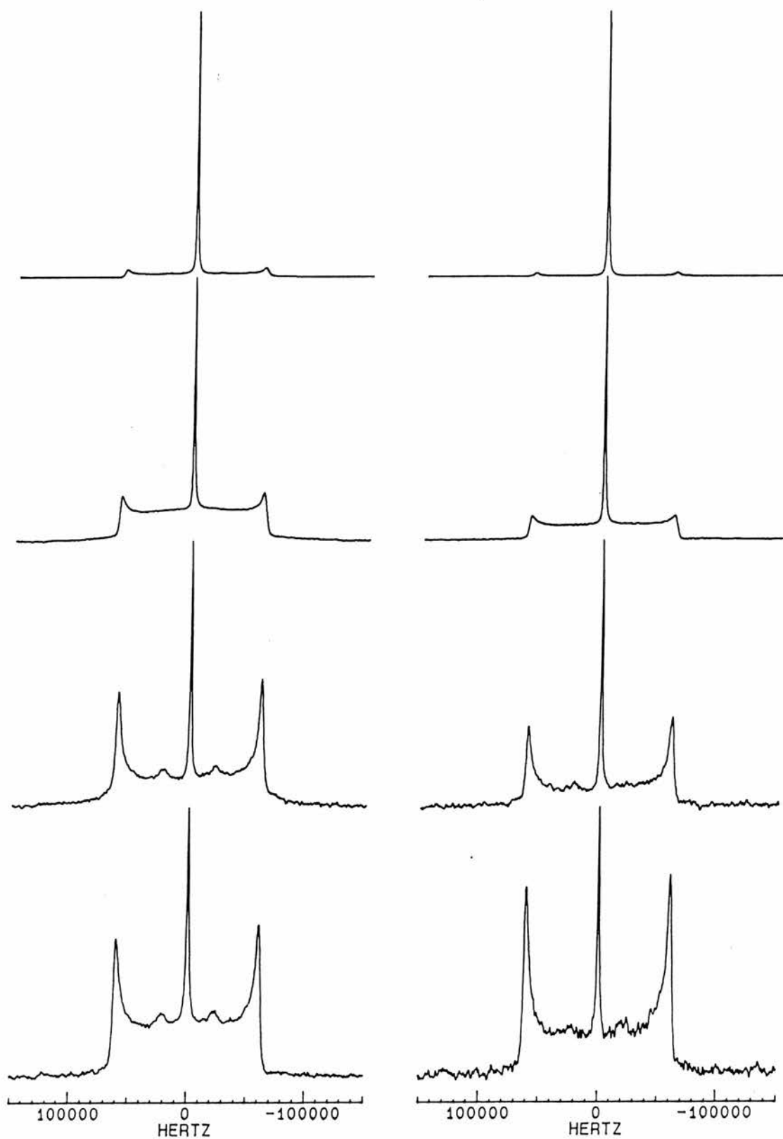
Figure 5.22. Measured ^2\text{H} quadrupolar echo spectra for 2,2,5,5- d_4 -hexane-1,6-diyl dibenzenesulfonate at different temperatures. Refocusing delay is 20 \mu\text{s} (left) and 160 \mu\text{s} (right). Temperatures are from top to bottom: 325, 288, 267 and 257 K.
