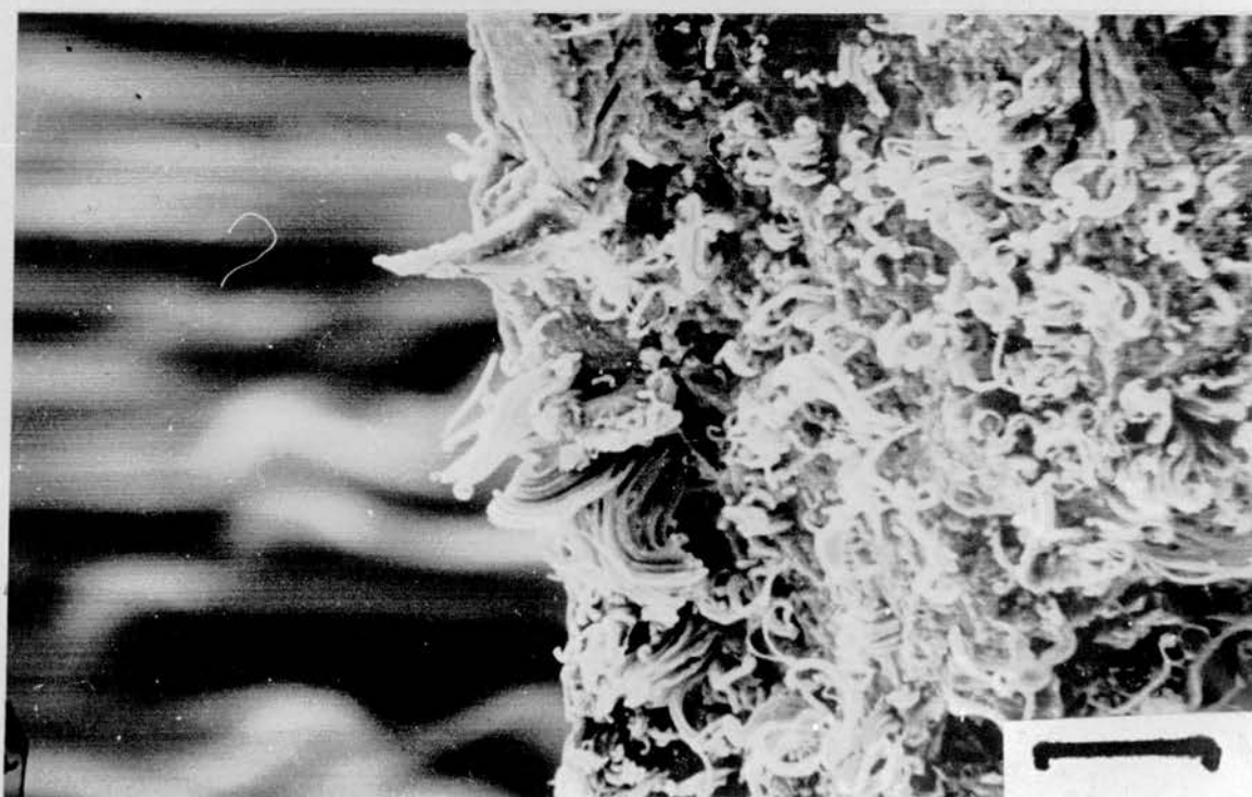
Plate 2: \text{Ag}_6\text{I}_4\text{WO}_4 electrolyte. No heat treatment. (20 \mu )
