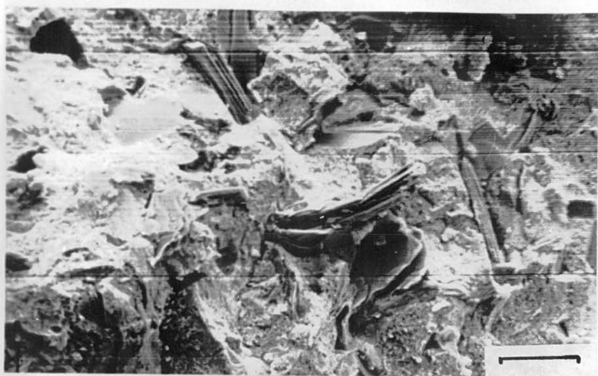
Plate 11: 290 0 C heat treated for 30 mins. (20 \mu )
