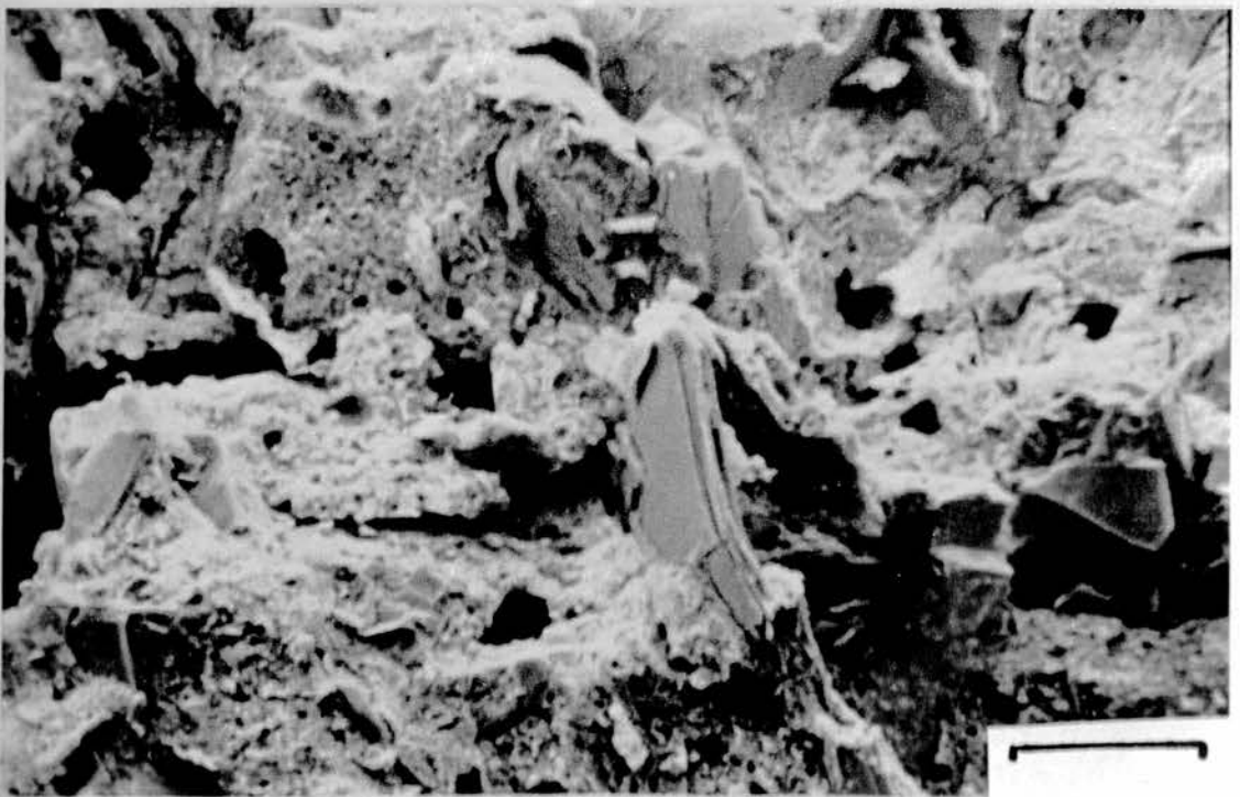
Plate 10: 300 0 C heat treated for 30 mins. (20 \mu )
