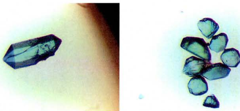
Fig.3.5.1.1 SSB crystals stained with IZIT dye. Right - a fragment of a hexagonal rod, Left - some degraded hexagonal bipyramids
