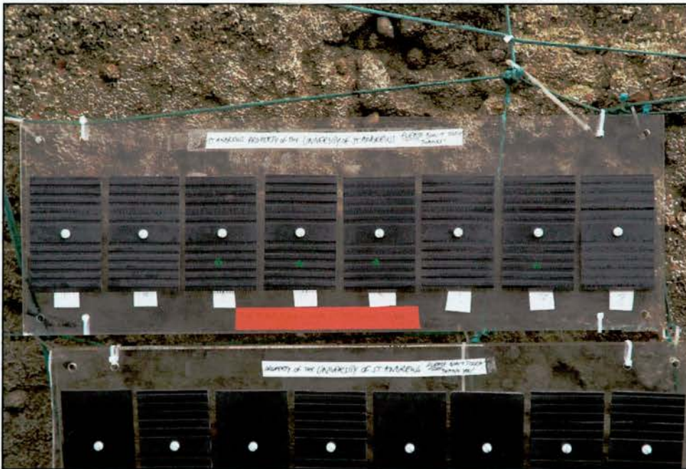
Fig. 29b – Site D at Kinkell Braes, 2002, showing latter panel configuration of four grooved panels with extract (*) and four grooved panels without extract (no star). This panel combination was used from the 11 th of May to the 2 nd of June. Backplates and mounting plates are 71.0 x 24.0 x 0.6cm clear acrylic sheets.
