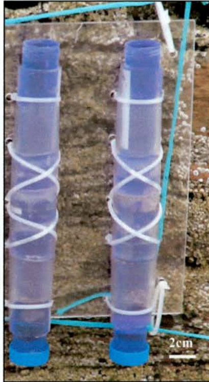
Fig. 16 – Larval traps containing 4M Urea 10ppm Bromophenol Blue solution, attached to backplate at Klingsbarns, 2002.
