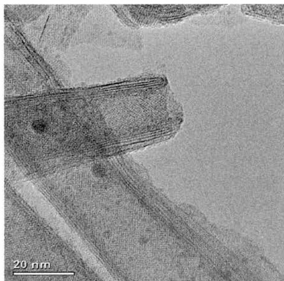
Fig. 4.3 TEM image of nanotube from K_{4-x}H_xNb_6O_{17} using butyl amine as an intercalating agent.
