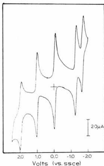
Fig 3.4. Cyclic voltammogram of [\text{Ru}_3\text{O}(\text{OAc})_6(\text{py})_3\text{BPE}]^+ at room temperature in 0.1 M TBAH- \text{CH}_3\text{CN} at scan rate of 500 mV/s.
