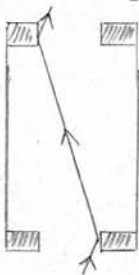
Figure 5. The effect of square aperture edges on the path of a ray of light.
