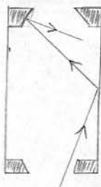
Figure 6. The effect of bevelled aperture edges of a sensitometer tube on the path of a ray of light.
