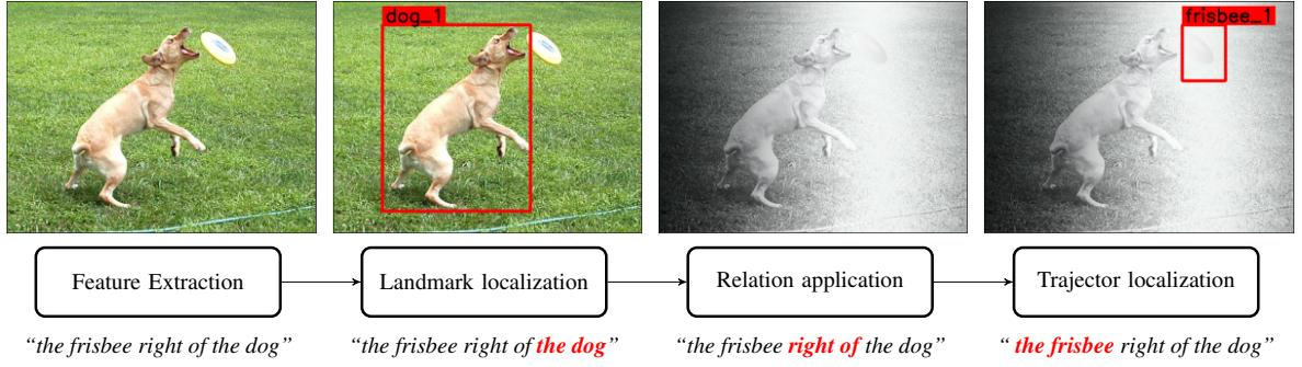
Figure 3: Example of the evaluation process for a single relation ““the frisbee right of the dog””. First, the model detects the appropriate landmark ““dog””, and generates the response map for the relation ““right of”” using the detected object as the landmark. Finally, the model detects the trajector ““frisbee”” and calculates the mean value of the response map of the bounding box.
