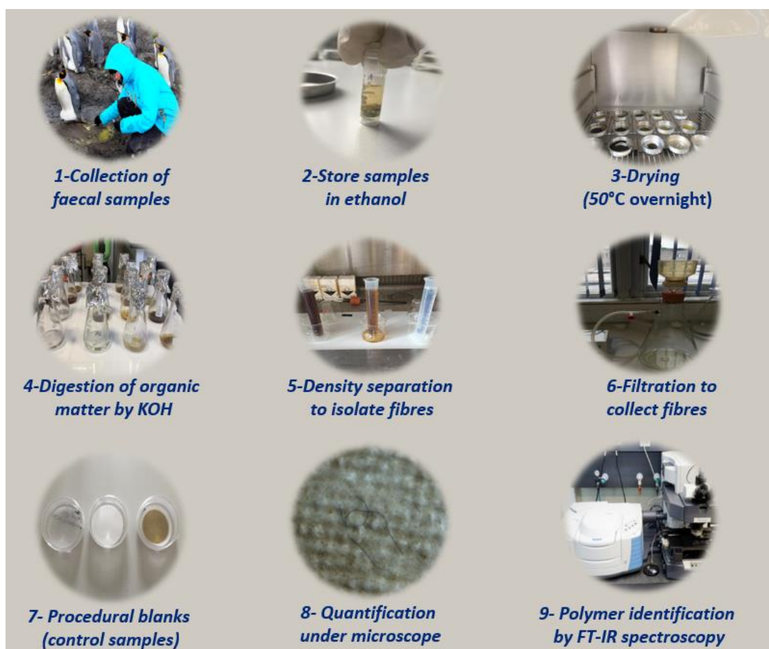
Figure 5.1. Illustrations of the different steps of the extraction phase of microplastics present in penguin faecal samples.
