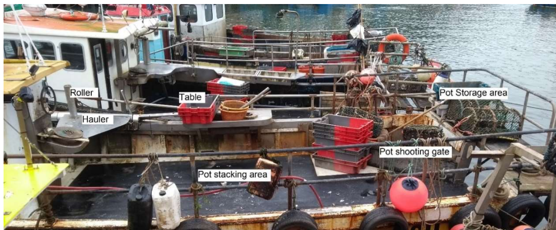
Figure 2. Examples of creel vessels and the layout of hauling equipment and key operating areas.
