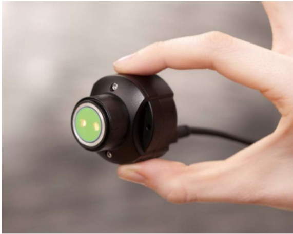
Figure 40. An example of a fibre optic accessory NIR measuring unit (O'Brien et al, 2012).
