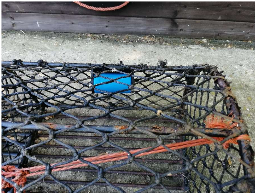
Figure 56. The ZebraTech WetTag; the blue cylinder at top of picture, installed in a creel.
