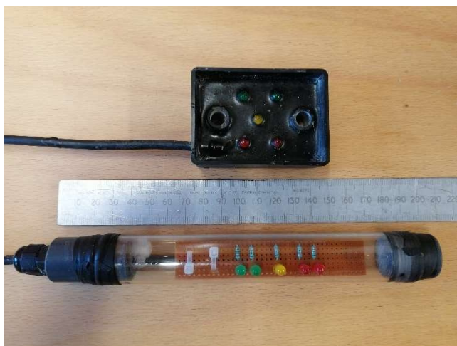
Figure 47. LED feedback panels, original polycarbonate (lower) and potted resin version (upper).
