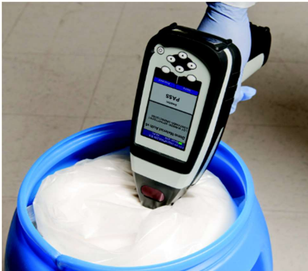
Figure 41. A handheld microPHAZIR™ RX Analyser for use in pharmaceutical industries (Thermo Scientific™, 2017).
