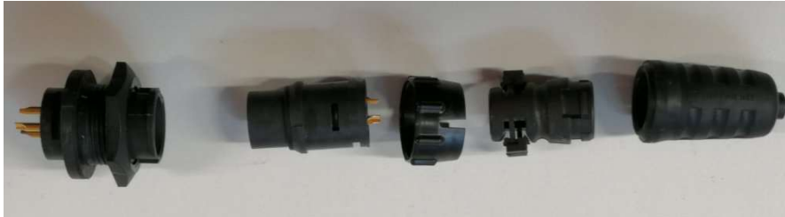
Figure 6. Original IP67 connector assembly.
