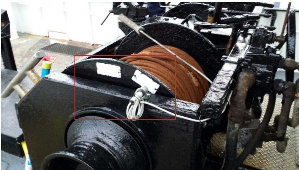
Figure 12. a winch sensor and reflectors fitted aboard a commercial Nephrops trawl fishing vessel (Course et al, 2015).
