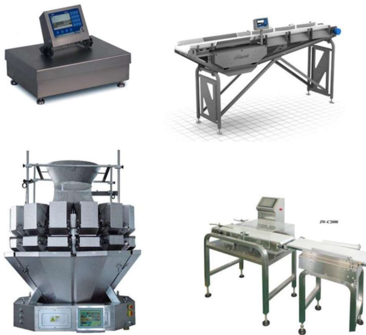
Figure 42. A selection of different weighing solutions investigated online. Includes motion compensating platform scales (Marel 2017a), in-line conveyor scales (Marel 2017b), hopper scales (Tecnimodern, 2017) and in-line scales with air jets that “blow” items on different pathways based on individual item weight (Food MC, 2017) (clockwise from top right).
