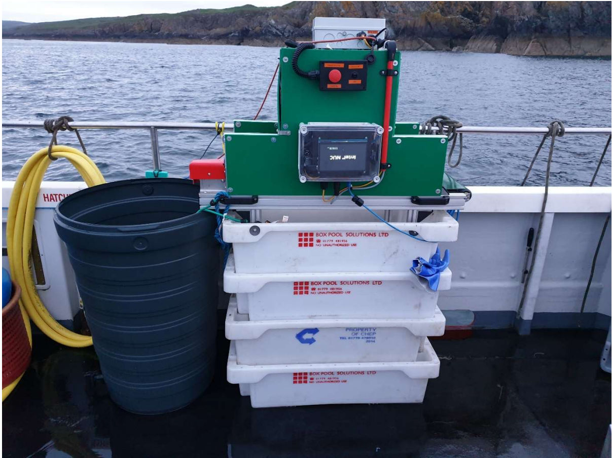
Figure 55. The completed ASSSID conveyor system on board the trials vessel.
