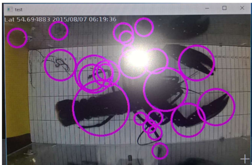
Figure 26. Haar Classifier output from field footage, note poor classification of some object areas.
