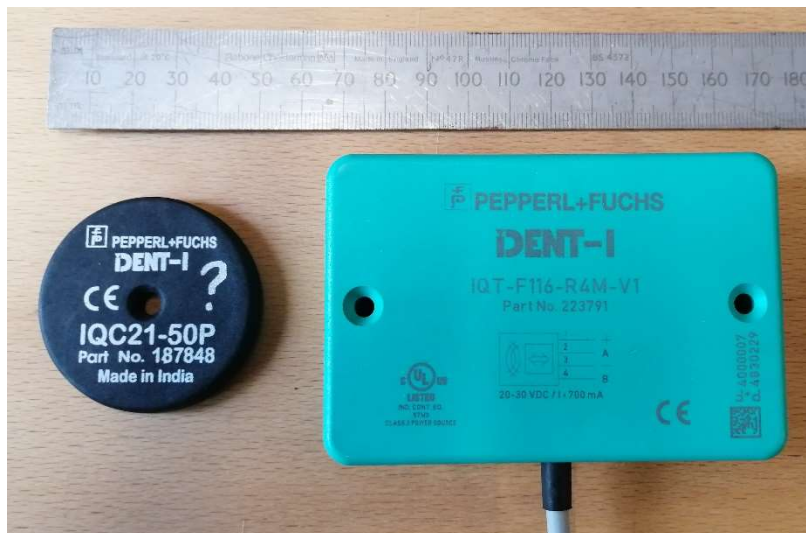
Figure 46. RFID reader head (right) and associated tag (left).
