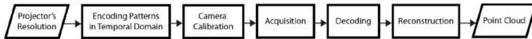
Figure 35. The step process required in the construction of virtual 3D objects utilising structured light scanning (Herakleous K and C Poullis, 2014).
