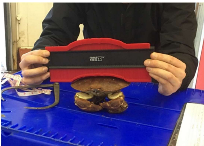
Figure 62. Measuring the dome height of a brown crab with a profile gauge.
