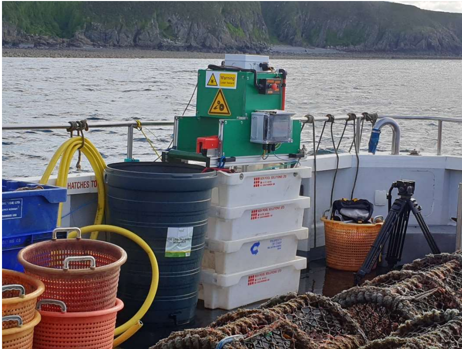
Figure 79. The ASSSID system and the water butt with a suspended fish basket inside, to catch animals undamaged once they have been scanned.
