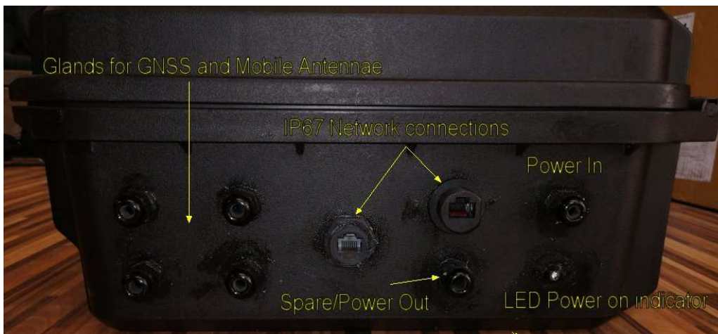
Figure 9. The end panel of completed logger unit, showing gland connection options along with panel mount LAN connections.
