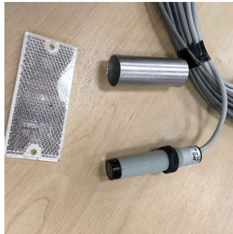
Figure 11. A winch rotation sensor with an attachable reflector.
