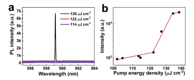
**Figure 2.** (a) Emission spectra of the single crystal laser on 350 nm grating. The spectra are shown for a pump energy below, at, and well above the lasing threshold. (b) Input-output characteristics of the same sample.
