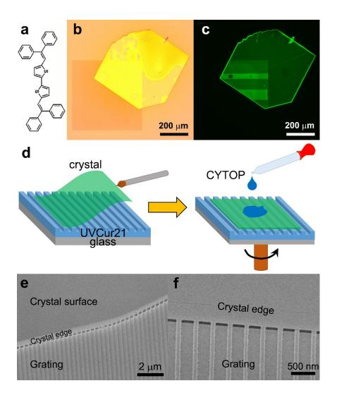
**Figure 1.** (a) Chemical structure of BDPV2T molecule. (b) Bright field image and (c) fluorescence image of an individual BDPV2T crystal on UV-NIL grating. (d) Schematic diagram of the sample fabrication. (e) 45° tilted and (f) 30° tilted SEM images of an individual BDPV2T crystal on top of 350 nm period linear gratings.
