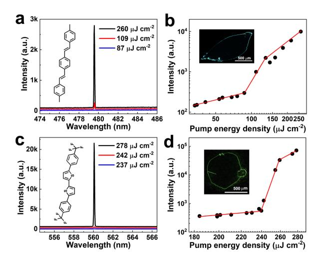
**Figure 4.** (a) Lasing spectra and (b) input-output characteristics of DSB-Me crystal on the 290 nm 1D linear gratings. (c) Lasing spectra and (d) input-output characteristics of P2T-CF<sub>3</sub> crystal on the 340 nm 1D linear gratings. Insets in b and d show fluorescence microscopy images of the respective sample.
