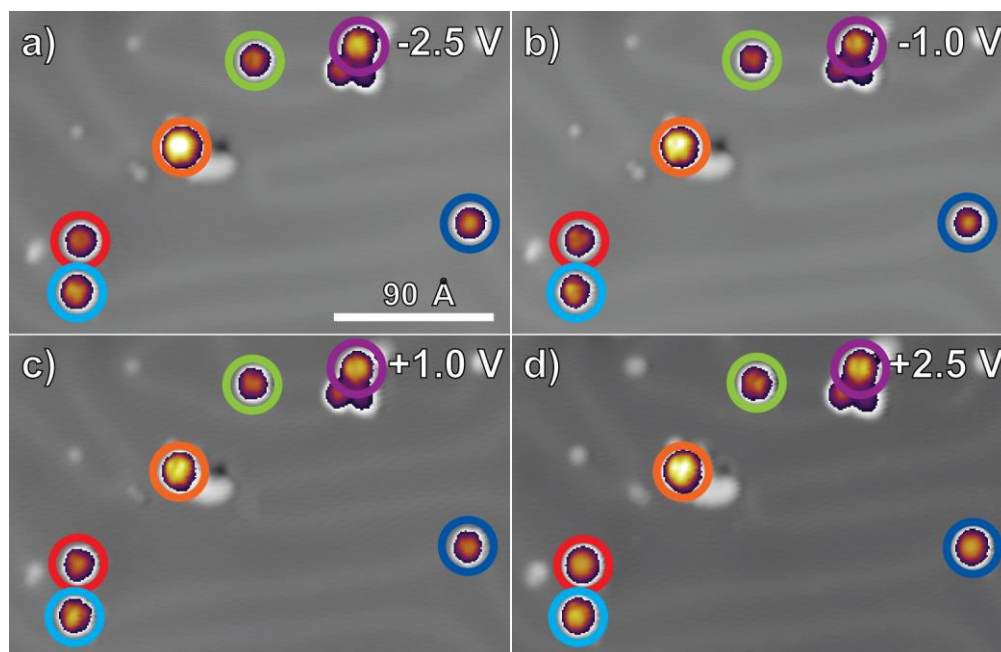
Figure 4.19: STM images of six isolated fullerenes on Au(111) after annealing at 320 K. a) (-2.5 V, 0.1 nA), b) (-1.0 V, 0.1 nA), c) (+1.0 V, 0.1 nA), and d) (+2.5 V, 0.1 nA).
