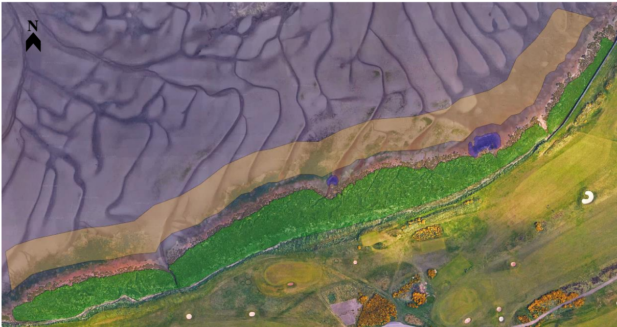
Figure 4.1: Aerial image of south shore of the Eden Estuary where sediment core sampling was conducted. Bottom right corner shows the edge of the Links Trust golf course. Semi-transparent polygons define the extents of each area type sampled. Brown is the mudflat; blue is the restored area of B. maritimus and green is the natural P. maritima marsh.
