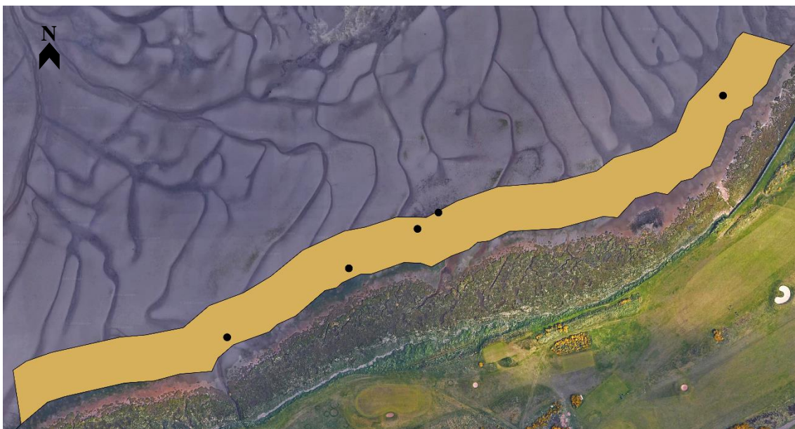
Figure 4.2: Aerial image of estuary showing polygon of mudflat area studied in brown. Black dots are location of core samples, located through random selection by QGIS .
