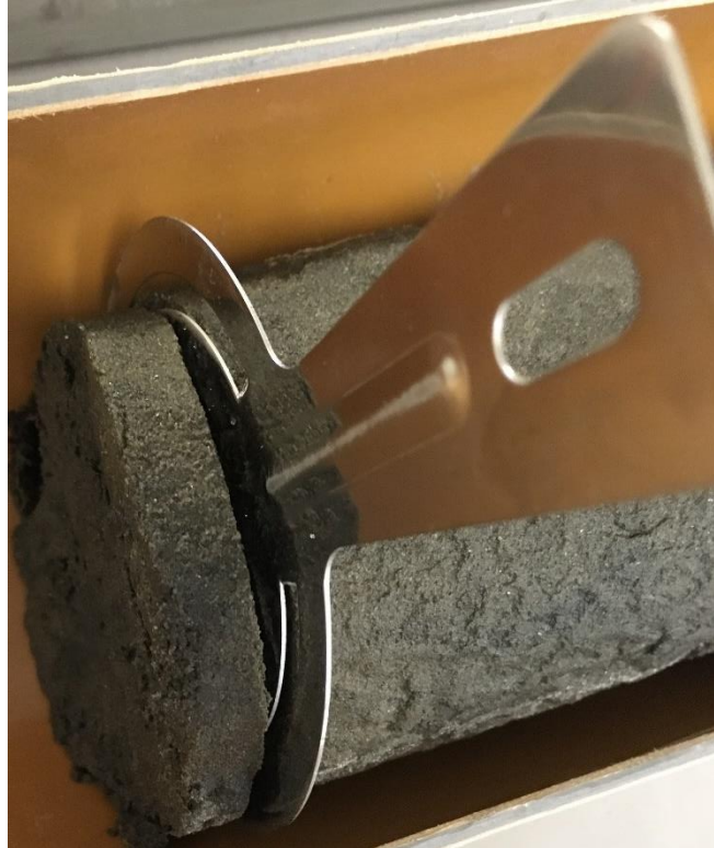
Figure 4.8: Sediment core being sliced with the sharpened disc core slicer. Showing a 1 cm section being removed.
