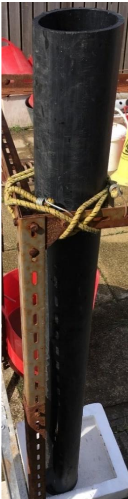
Figure 4.6: Thick walled pipe section which was filled with hot water and used to rapidly heat frozen core tubes, facilitating the removal of the sediment core.
