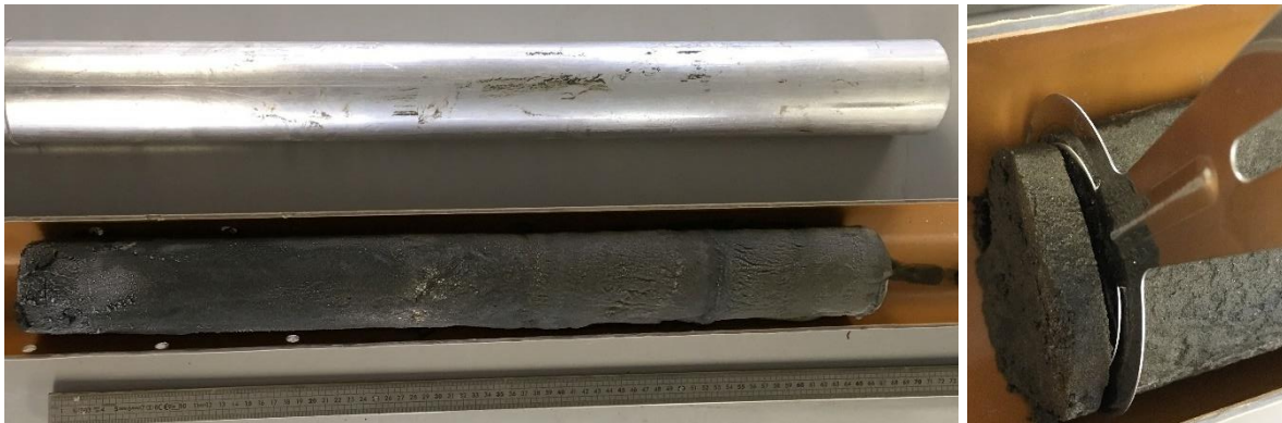
Figure 1.17: Left image of sediment core retrieved from core tube and right image shows top of core being sectioned into 1 cm layers.
