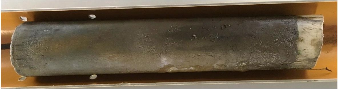
Figure 4.7: Frozen sediment core after extraction from core tube into half-pipe capture device. Showing retained head of excess water (right, whitish block) held above the sediment during collection.
