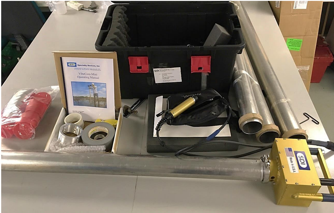
Figure 4.5: A hand-held Vibecore-Mini unit with a 4-inch core tube attached. Along with additional core tubes and accessories.
