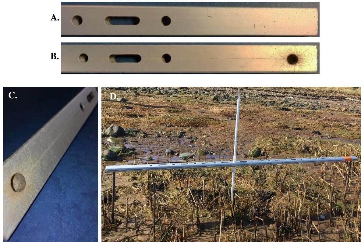
Figure 3.8: (A) Top of the 'table' bar, circular holes used as measurement points. (B) Underside of 'table' bar, right hole used to attach to rods. (C) Showing depth of attachment hole of the 'table'. (D) Showing SEB being used to measure sediment elevation in the environment.
