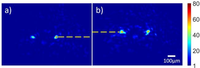
**Fig. 3.** Example of the NL-OMEM through nonlinear perturbation. Using a pump power of 150mW at a distance of 0.53mm from the pump. Left: Original wavefront. Right: Perturbed wavefront exhibiting the NL-OMEM.
