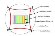
Diagram 1. Structure of IPD Detector
