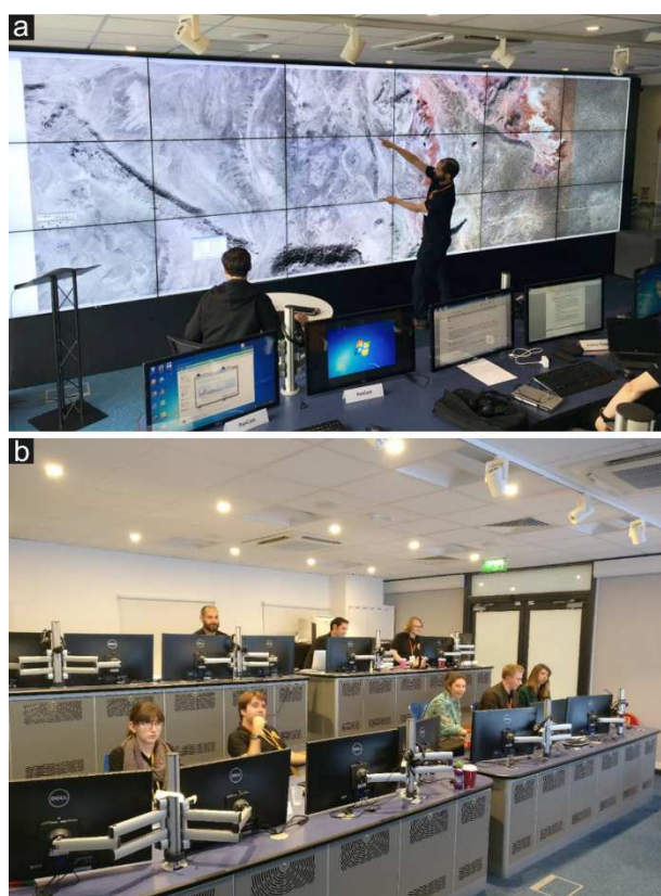
325 326 Figure 5. MOC setup. a) The large video wall. The desktop view of one workstation could be stretched 327 over the whole wall, as here, or several workstation desktops could be split across the screen ‘on the 328 fly’. b) The tiered workstations for the SWT stations. Image credit: Andrew Griffiths.
