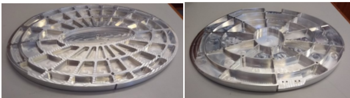
Figure 4. Dragonian focusing mirrors showing stiffening ribs on rear of static secondary mirror (left) and reciprocating primary mirror (right). The focusing surfaces conform to the design profile within \pm 30 \mu\text{m} ( \sim \lambda/30 ).
