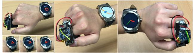
Figure 13: (left) Gestures recognizer for shortcut commands, (middle) 2D map navigation, (right) Analog clock.
