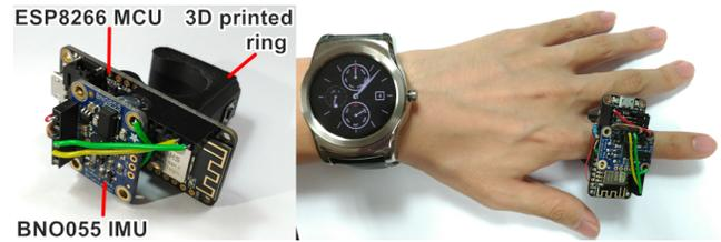
**Figure 1: (left) Assembled custom smart ring device (right) when worn on finger together with an Android smartwatch.**
