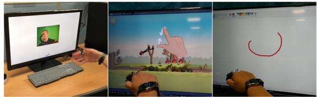
Figure 14: Example applications on the PC: (left) Swiping game (middle) Angry bird and (right) MS Paint application.
