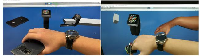
**Figure 2: (left) Initially we tried with a smartphone imitating a ring and controlling primitive blocks. (right) Trying with a custom assembled ring and controlling a 3D hand model.**
