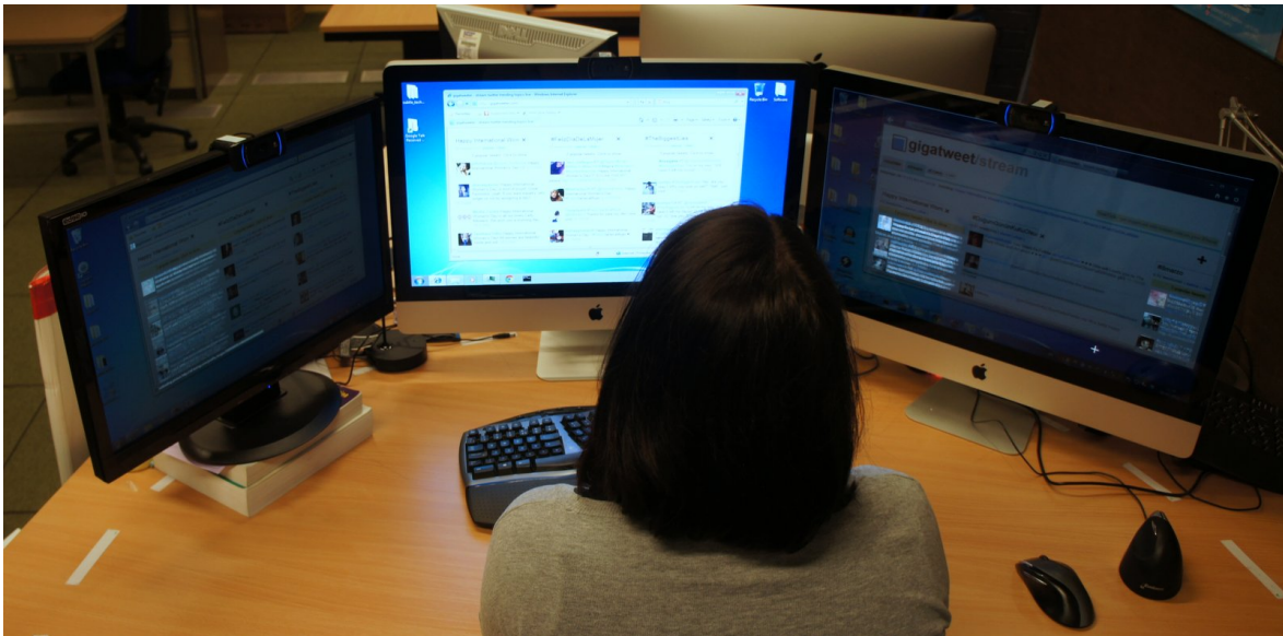
Figure 7.1: An illustration of one of the techniques for visualising changes on unattended displays in action on the two peripheral displays. The PixMap technique highlights any pixels that change as a temporal heatmap.
