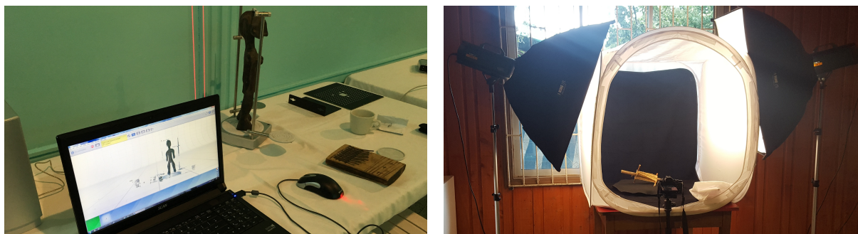
Figure 7.1: Digitising an artefact using a laser scanner (left) and photogrammetry (right)
