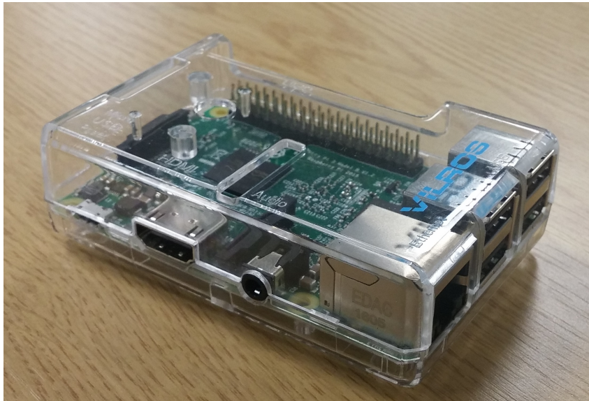
Figure 6.4: Raspberry Pi in a transparent plastic case
