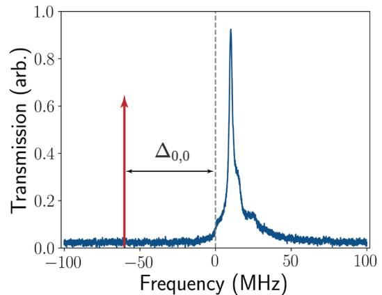
FIG. 1. Transmission spectrum of the employed near-confocal cavity. All data in the main text are taken with detuning  $\Delta_{0,0} = 60$  MHz, defined from the position of the  $\text{TEM}_{0,0}$  resonance.
