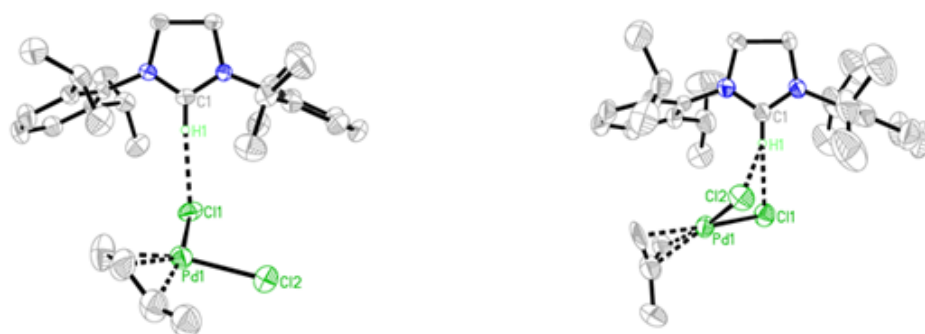
Figure 5.4: Single crystal structure of Pd(ate)-10 (left) and Pd(ate)-11 (right)
