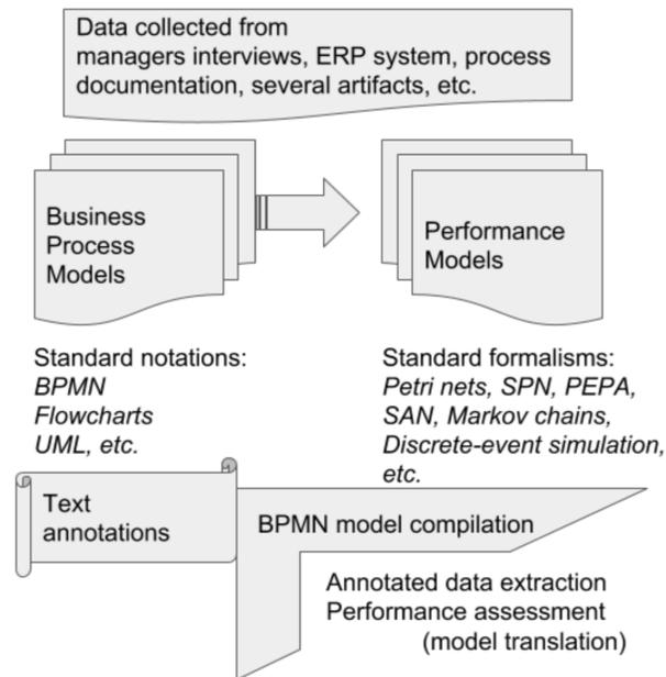
**Fig. 1.** Interplay between process models and performance models
