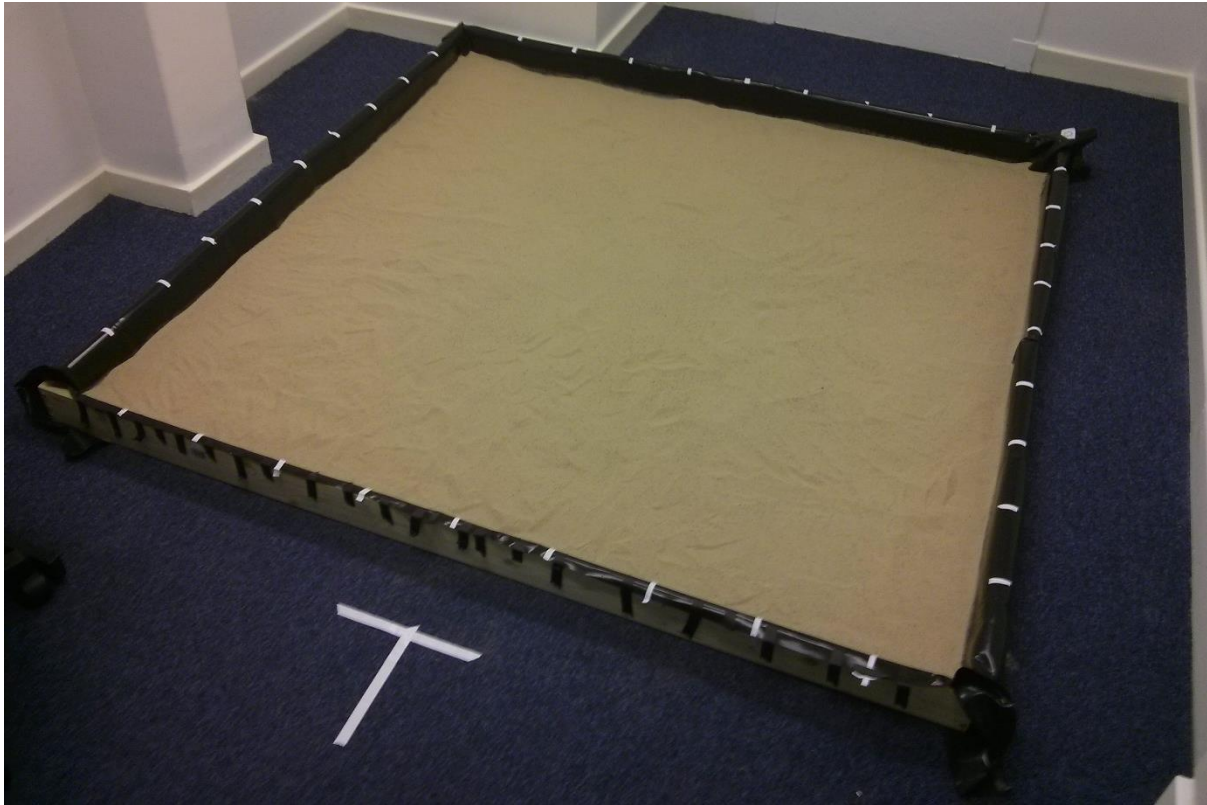
Figure 9.12: Photograph of the sandpit used to hide real world objects in. Note the white markers around the edge, and the T shaped tape on the floor that the participants stood with one foot each side of the stem.
