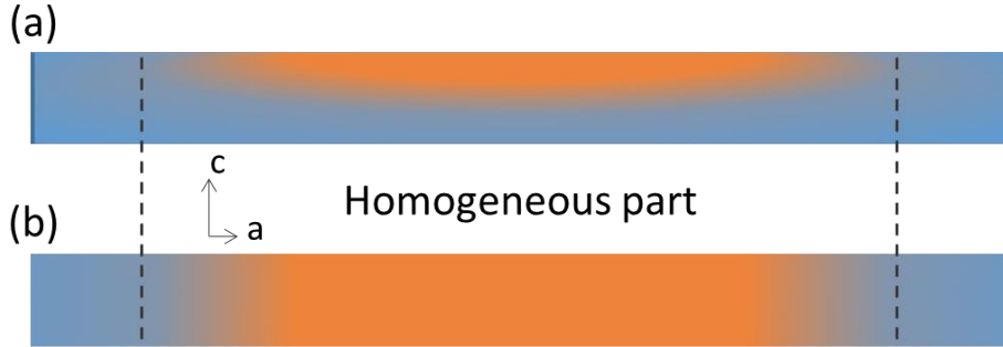
Figure 3.30: Schematic diagrams for heat flows (a) from c -axis and (b) from b -axis. The dashed lines indicate the homogeneous region of the sample.
