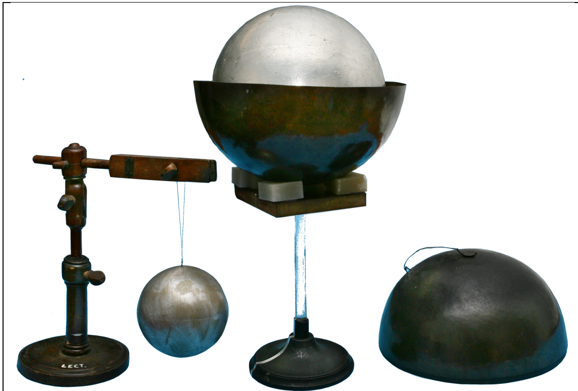
Figure 2. Maxwell and MacAlister's apparatus. The additional ball hanging from the retort stand has traditionally been considered part of the apparatus, but does not correspond to the brass ball for testing sensitivity of Maxwell's description. Photograph courtesy of the Cavendish Laboratory, Cambridge.
