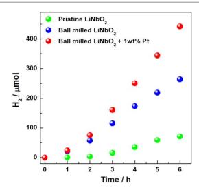
**Figure 2.** Time-dependent photocatalytic hydrogen evolution from pristine LiNbO<sub>2</sub>, ball-milled LiNbO<sub>2</sub> and ball-milled LiNbO<sub>2</sub> with 1 wt% Pt. Measurements were performed upon 0.2 g powders in 200 ml oxalic acid aqueous solution (0.025 M). Light source: 250 W iron doped metal halide UV—vis lamp with a UV cut-off filter ( $\lambda \ge 420$  nm).
