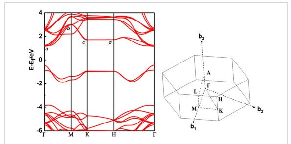
Figure 3. Calculated band structure of LiNbO<sub>2</sub>, energy zero point was set at Fermi level. Brillouin zone for a hexagonal lattice was shown on the right.
