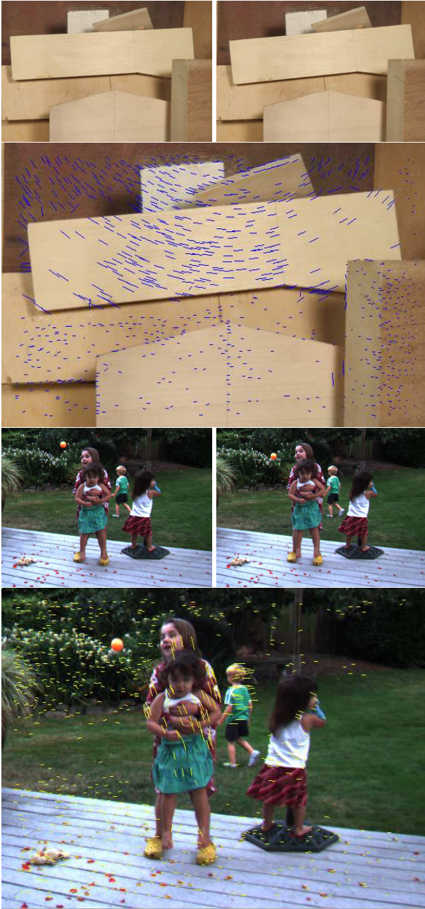
Figure 11: Example of optical flow determination using our keypoints and keypoint descriptors. Rows 1 and 3 show two successive frames from two different sets. Rows 2 and 4 show the optical flow results obtained from matching keypoints between the two frames. The images belong to the Middlebury Optical Flow dataset (Scharstein, 2009a)
