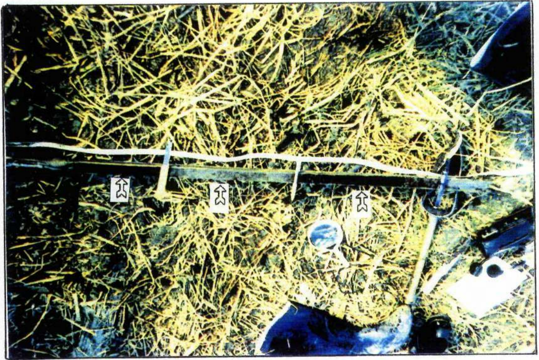
c). Sediment Inside a Gouge Sampler Showing Two Peat Layers Separated by a Minerogenic Layer at Panigati (Photograph by the author)
