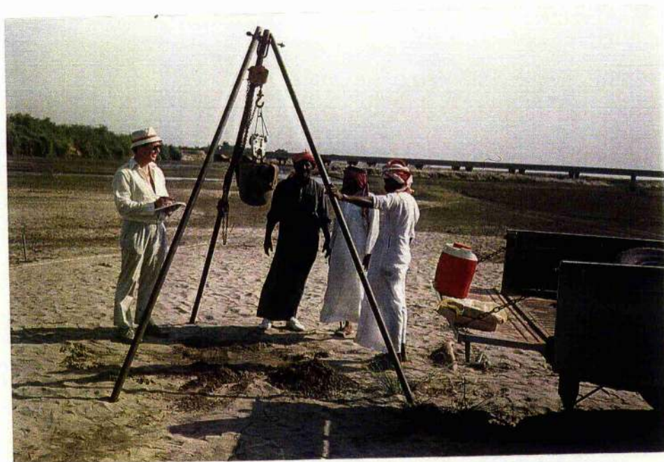
Figure 6.7 Surveying team using a heavy weight dumper (70 kg) to generate energy at a seismic station in the middle part of Wadi Baysh.
