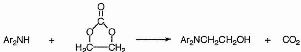
Scheme 5.11 Synthesis of the N -(2-hydroxyethyl) diphenylamine
