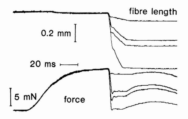
Fig. 3. a) A typical trace from a slack test performed on a myotomal preparation from the saddle wrasse (Thalassoma duperreyi). Stepwise length changes (AL) were given during the plateau phase of the tetanus to drop the force generated to zero. b) AL was plotted against the time required to take up the slack and begin to generate force (AT); unloaded contraction velocity was determined from the slope.
