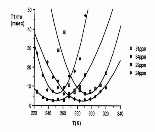
Figure 3.6: T<sub>1</sub> $\rho$  versus temperature for the *t*-butyl carbons of (4)
