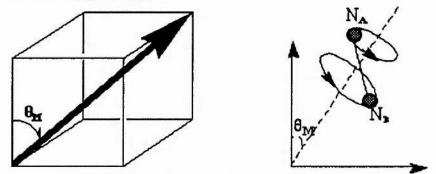
Spinning the sample about  $\theta_M$  averages the direction of all the NA/NB interactions. The average of the vector AB is the magic angle.
