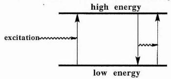
Since there are more nuclei in the lower energy state, the effect of both these processes results in a net absorption of energy and the NMR spectrometer registers this absorption plotting it as a peak in the spectrum.
