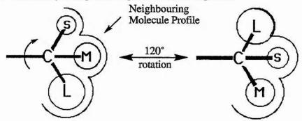
If there is an unsymmetrical group as in figure 1.13, then the distress caused to the lattice as the large group L passes through the position occupied by small group S will be large. Such a rotational process is, therefore, most likely to be observed when the rotating group approaches conical symmetry.
