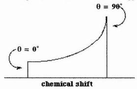
These effects, dipolar coupling and chemical shift anisotropy, are not observable in solution NMR as the rapid molecular tumbling averages the dipolar vectors and the anisotropy to zero. This decouples the magnetic nuclei by the rapid changing of their orientations and leads to a single isotropic chemical shift.
