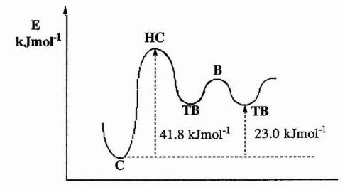
The energy difference of 23 kJmol<sup>-1</sup> between the chair and twist boat forms ensures that cyclohexane exists almost exclusively in the chair form at room temperature.
