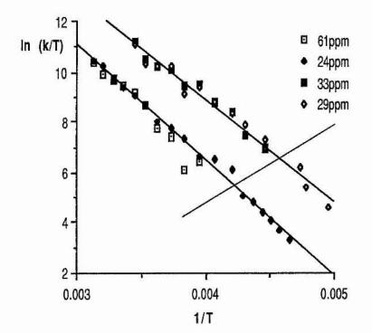
This data can be used to determine the enthalpy and entropy of activation for the rotation of the *t*-butyl groups. The relevant equations are:
