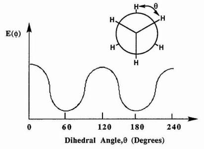
Figure 1.11: The Potential Barrier to the Rotation of Ethane.
