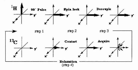
Figure 1.8: The Cross Polarisation Pulse Sequence.
