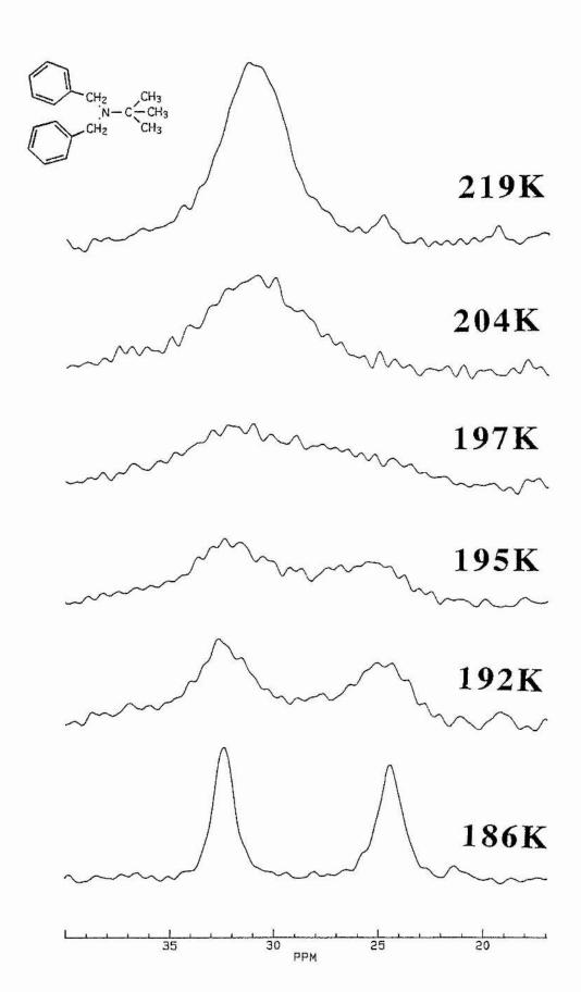
Figure 3.26: Variable Temperature <sup>13</sup>C CP/MAS Spectra of the *t*-Butyl Group of Compound 9(b)
